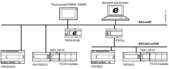
The PXG3.W100 web interface serves as the central access point to operate the automation level. A central access point also allows for concurrent operation of different operator units while supporting connection of the Desigo touch panels PXM40 / PXM50 as well as providing access using devices featuring a standard web browser. The following functions are available to operate and monitor a plant:
