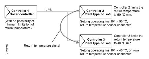
The zone controller with its own return temperature sensor (plant type 4 - x) passes the return temperature to the other zone controllers in the same segment. These can thus ensure minimum limitation of the return temperature locally, depending on the settings made, which means that they generate a critical locking signal internally. (For response to critical locking signals, refer to chapter 17.4.5 "Locking signal gain").
