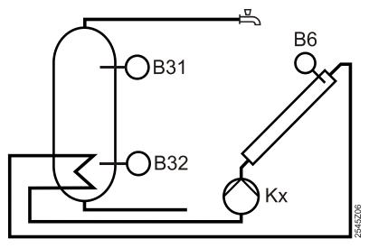
B31 Storage tank sensor 1 B32 Storage tank sensor 2
