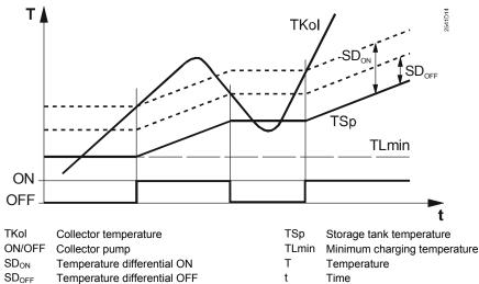
• The storage tank is charged when the collector temperature exceeds the current storage tank temperature by the switch-on differential:
