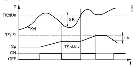
TSpSi Maximum limitation storage tank temperature
