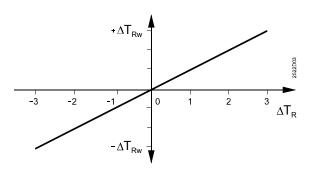
The flow temperature setpoint change  $\Delta T_{Vw}$  resulting from the change of room temperature setpoint is calculated as follows:
