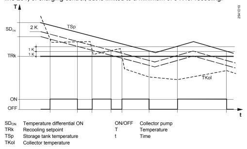
If the storage tank temperature lies at least 2 K above the recooling setpoint and by at least the temperature differential ON above the collector temperature, the collector pump is activated:
