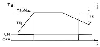
TSp Storage tank temperature T T Temperature TSpMax Maximum limit value of charging temperature t Time
