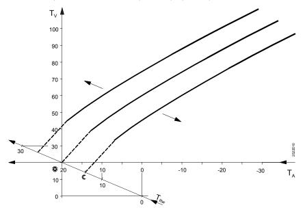
Parallel displacement of heating curve
