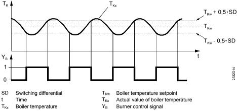
Note on setting: When controlling a 1-stage burner, the reset integral of the second stage should be set to zero.
