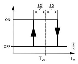
ON Actuator operating OFF Actuator dead
