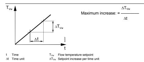
The rate of increase of the flow temperature setpoint can be limited to a maximum (heating up brake). In that case, the maximum the flow temperature setpoint can increase is the set temperature per time unit (°C per hour). This function ...
