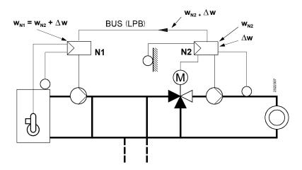
N1 Boiler temperature controller (heat generation)
