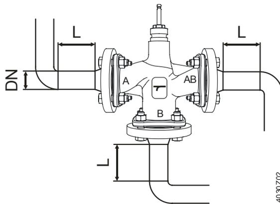
$L \geq 0.4 \text{ m} \dots \geq 10 \times \text{DN}$
