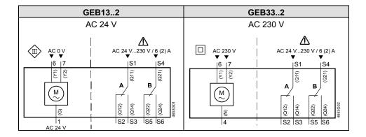
**Modulating control** Y = DC 0...10 V, 2...10 V, 0...35 V
