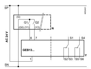
NControllerYActuator GEB13..2SPSystem potential AC 24 VSNSystem neutralQ1, Q2Controller contacts
