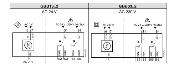
Modulating control Y = DC 0...10 V, 0...35 V
