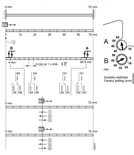
The setting shafts for the auxiliary switches turn together with the actuator. The scales are valid only for the **zero position of the actuator** (push rod retracted) on **"outward"** linear travel.
