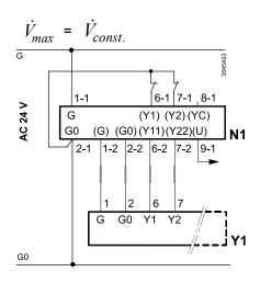
Modulating control  $\dot{V}_{max}$  and  $\dot{V}_{min}$  and complete shutoff and fully open operating mode "con"
