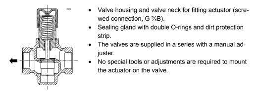
**Manual adjustment** The valve can be adjusted manually from 0...100 % by use of the plastic manual adjuster (which also acts as a protective cover during transport).
