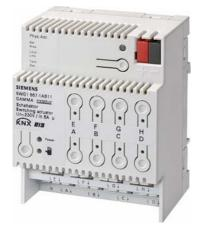
The switching actuator N 567/11 is an N-type device for DIN-rail mounting. With its eight relay contact outputs (channels) it can switch eight groups of electrical consumers independently of each other. The connection to the bus line can be carried out either via a bus terminal block or by a contacting system to a data-rail installed in the DIN-rail.
