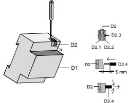
Figure 3: Connecting and disconnecting the cable
