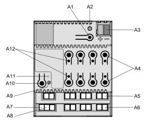
Figure 1: Location of the display and operating elements
