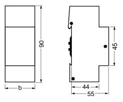
b = 4 module units (1 module unit = 18 mm)
