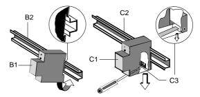
Figure 2: Installing / dismantling the DIN rail mounted device
