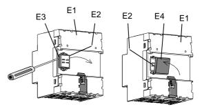
Figure 4: Covering the contact system
