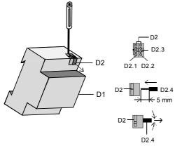
Figure 3: Connecting and disconnecting the cable
