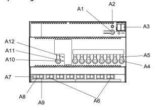
Figure 1: Location of the display and operating elements
