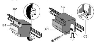
Figure 2: Installing / dismantling the DIN rail mounted device
