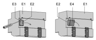
Figure 4: Covering the contact system
