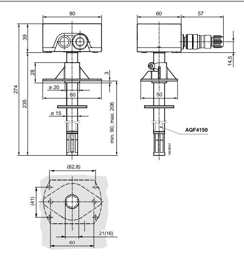
Drilling template with (without) mounting flange
