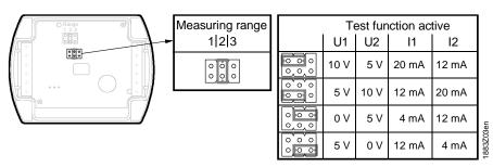
The setting element is located inside the cover. It consists of 6 pins and a shorting plug. It is used for selecting the required temperature measuring range and for activating the test function.
