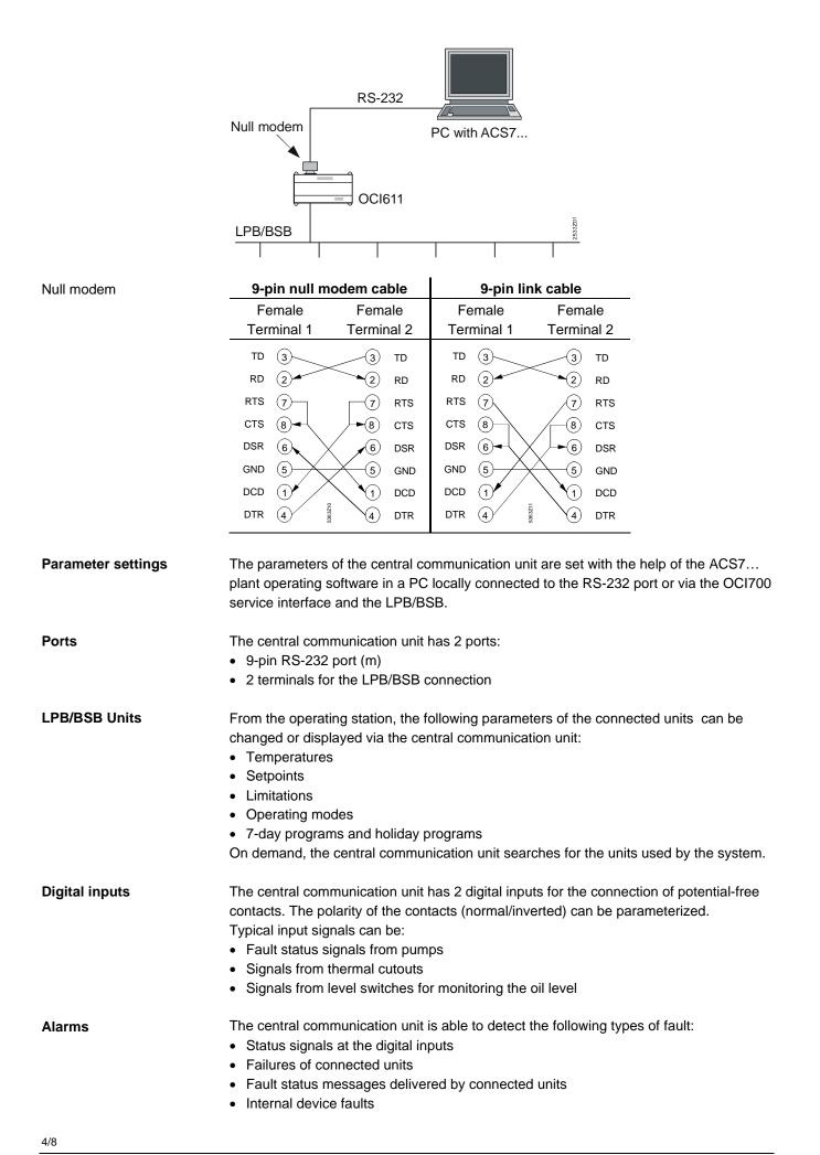
For each alarm source (central communication unit, digital inputs, LPB/BSB), it is possible to select whether its alarms shall be delivered only when they occur, or when they occur and disappear.
