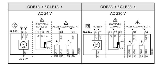
Modulating control Y = DC 0...10 V, 0...35 V
