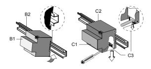
Figure 2: Installing / dismantling the device
